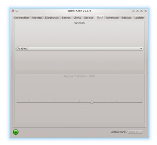
Rescue mode complements the normal operation of the Spirit unit. If activated, the model will recover to a configured inclination and can start with ascending as per the settings. This function can be used any time when the pilot loses orientation or control of the model.
