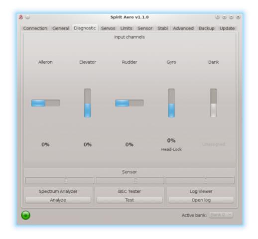
i) For proper operation of the unit, it is necessary that movement of each channel correspond with the bars. Direction of the movement must be same as well.
