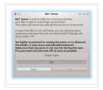
Click the *Start* button to start the test. After 20 seconds it should be finished. If you will observe any issue, then your power supply is insufficient and should not be used. In this case power supply with higher current rating should used.
