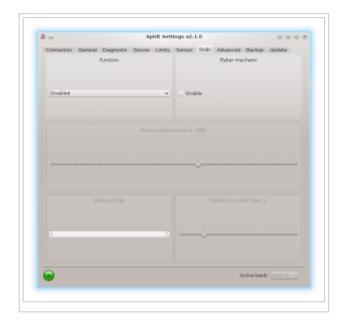
Rescue mode complements the normal operation of the Spirit unit. If activated, the model will recover to a horizontal position and add collective pitch as per the settings. This function can be used any time when the pilot loses orientation or control of the model.
